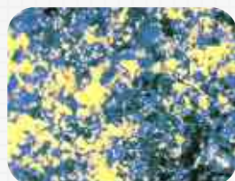
Shell microstructure comprising Bainite Magnification : 500 X
