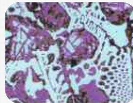
Shell microstructure comprising Bainite Magnification : 500 X
